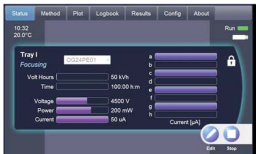
Typical current pattern on tray 1 displayed online during OFFGEL fractionation.
